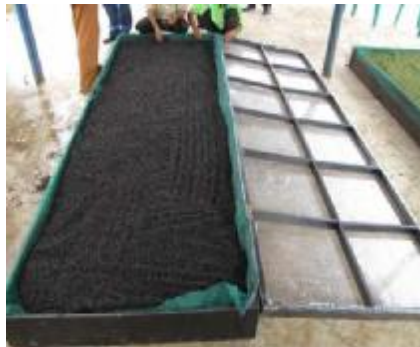
Gambar 7. Contoh alat pengering energi sinar matahari (solar dryer)
